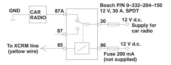
Another possibility is to use a special muting unit, which mutes the radio by connecting load resistors to the speaker lines of the car radio. Bosch P/N 0-332-204-150
